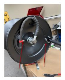
ONCE THESE STEPS HAVE BEEN DONE, CRANK WITH THE HANDLE OF THE REEL TO SPOOL HOSE ONTO THE DRUM OF THE HOSE REEL.
